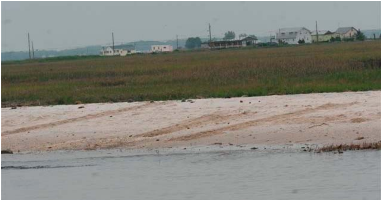
Photo 5 Trenches dug perpendicular to Gandy's Beach, approximately 17-20 m long. The sand-egg mixture was spread over a 2 m wide strip on the left side of the trench as shown in the photograph.
